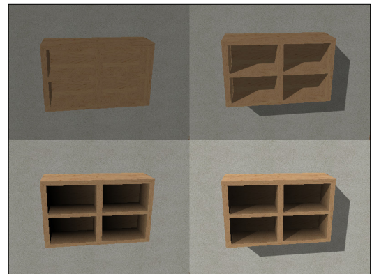
[Fig. 12] A rendering of book shelf model (76 tris.) (Top: using OpenGL fixed functions, Bottom: using SHL) (Left: without a shadow map, Right: with a shadow map)
