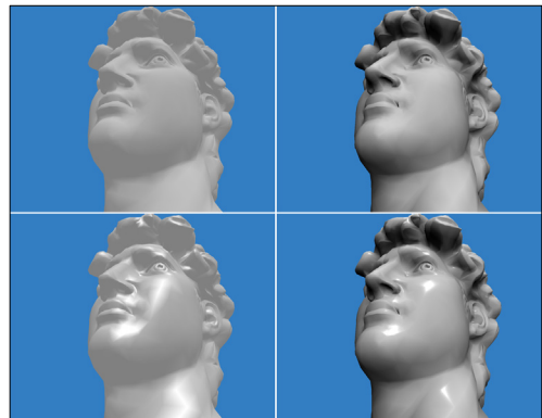
[Fig. 11] A rendering of David head (16,111 tris.) (Top: diffuse only, Bottom: with specular reflection) (Left: without SHL, Right: with SHL)
