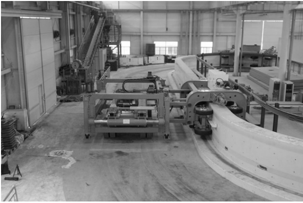
Fig. 5. Accelerated Pavement Tester
