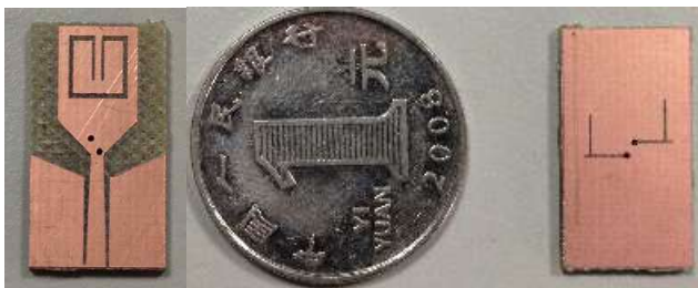
Fig. 8. Geometry of the fabricated band-notched UWB antenna
