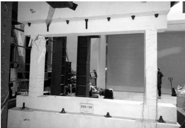
Fig. 14 Crack pattern (DSS-00)
