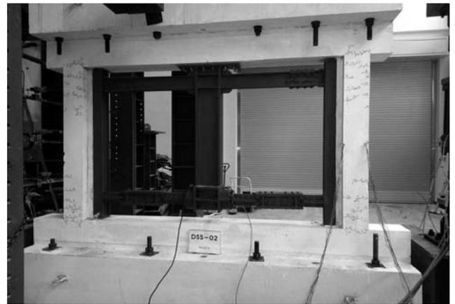
Fig. 15 Crack pattern (DSS-02)
