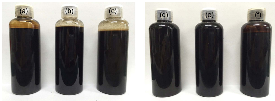
Figure 5. Phase separation behavior pictures of asphalt with (a) S4ID, (b) S5ID, (c) S6ID, (d) S4DD, (e) S5DD, and (f) S6DD.
