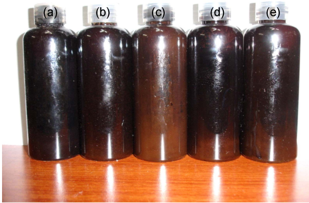
Figure 2. Phase separation behavior pictures of asphalt with (a) OA, (b) DA, (c) DDA, (d) ID, and (e) F-ST.
