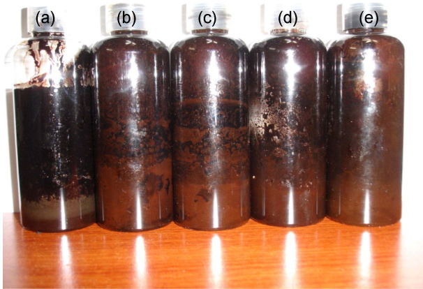
Figure 3. Phase separation behavior pictures of asphalt with (a) Tween 20, (b) Tween 60, (c) Tween 80, (d) Tri-200, and (e) Tri-5M.
