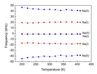
**Fig. 3.** (Color online) Zeeman splitting of NMR spectrum for  ${}^{23}$ Na in NaBrO<sub>3</sub> single crystal. The zero point is 52.9015 MHz.
