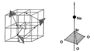
**Fig. 1.** Crystal structure of NaBrO<sub>3</sub> in the unit cell. The vertical line is the symmetric axis of the electric field gradient at the Na and Br sites.
