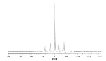
**Fig. 2.** Typical nuclear magnetic resonance spectrum of <sup>23</sup>Na nucleus at 300 K operating at  $\omega_o/2\pi$ =52.9015 MHz. The inner satellite line within ±30 kHz is denoted as Na(I) center, whereas the outer side ±30 kHz is denoted as Na(II) center.
