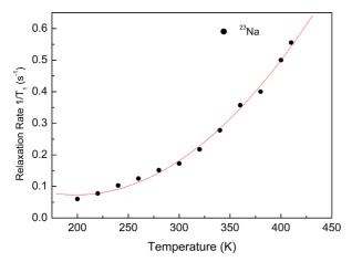
**Fig. 5.** (Color online) Temperature dependence of spin-lattice relaxation rate  $1/T_1$  for <sup>23</sup>Na in NaBrO<sub>3</sub> crystal. The solid line is fitted by assuming Raman processes.
