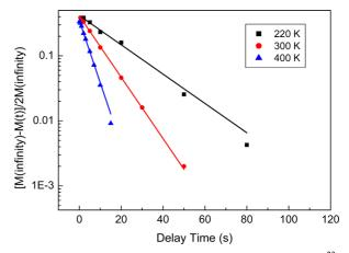
**Fig. 4.** (Color online) Magnetization recovery traces of  $^{23}$ Na in NaBrO<sub>3</sub> crystal as a function of delay time at several different temperatures. The solid lines are fitted using Eq. (1).
