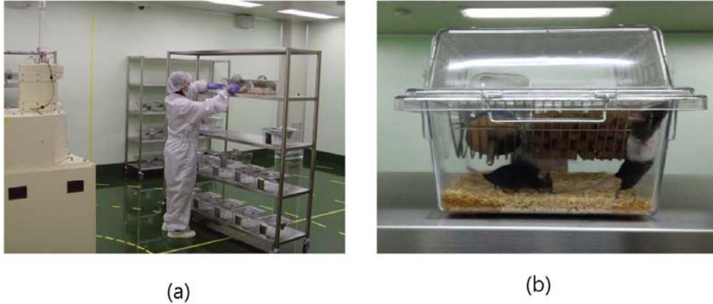
Fig. 1. Conventional irradiation method. (a) A shelf of irradiation apparatus: 420W × 205L × 185H mm. (b) Standard laboratory mouse cage: 200W × 260L × 130H mm (polycarbonate cage)
