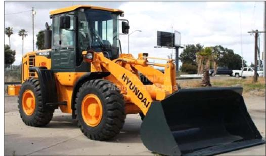
Fig. 12 Z-bar type wheel loader
