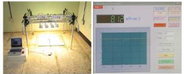
Figure 2. Accelerated experiments of color change using artificial light
