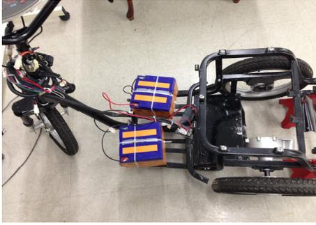
Fig. 6 Chassis of small electric vehicle
