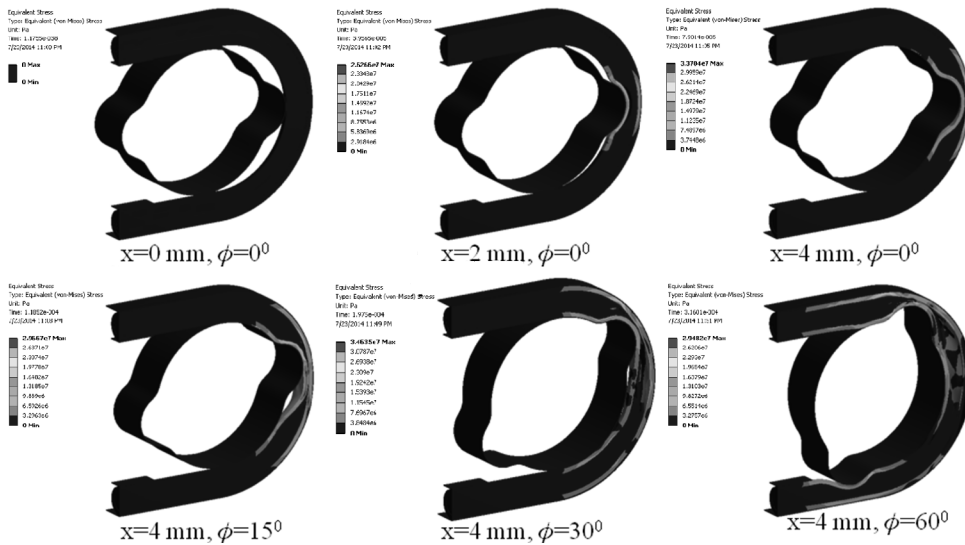
Fig. 13 Stress versus roller angle
