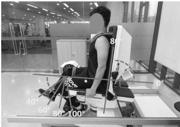
Figure 1. Experimental settings for the measurement of knee extension torque and hip-knee joint angles
