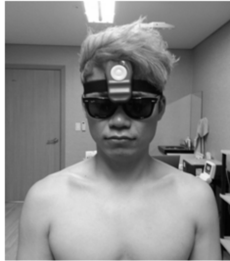
Fig. 1. Electrogoniometer attachment position
