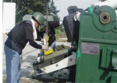
Figure 7. Laying on the loading device by hoist-type transfer system
