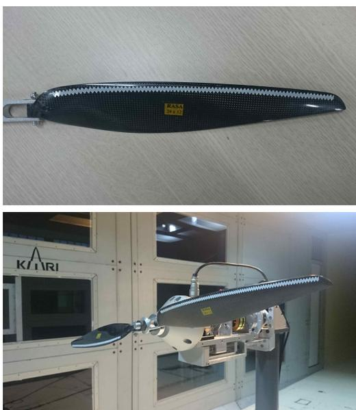
Fig. 8. 24" propeller with transition tape
