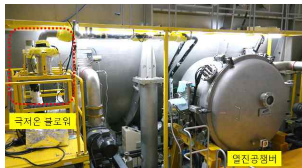
Fig. 14. Blower test configuration on thermal vacuum chamber
