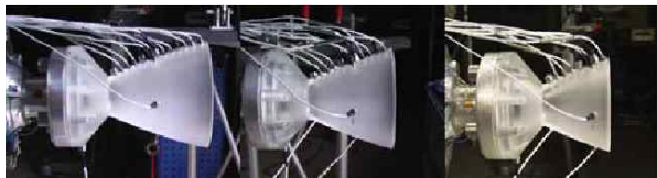
Fig. 11. Dual bell nozzles with different lengths for N 2 cold gas experiments[13]
