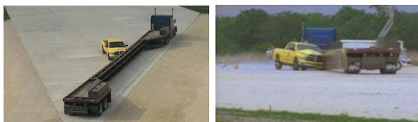
Fig. 1 Mobile Barrier Crash Test
