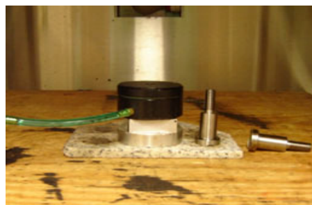
(b) Piston and Pull-Out Stubs in Chamber
