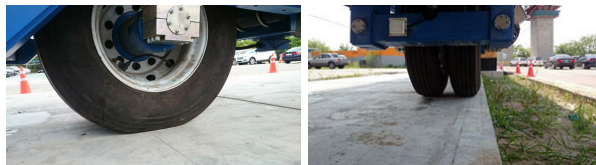
(a) Center Loading (b) Edge Loading
