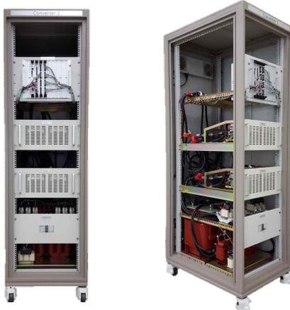
Fig. 10. 10kW reduced model of power system.
