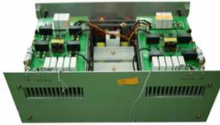
Fig. 7. Picture of developed 20kW EV fast charger block consisted of two 10kW converter modules.
