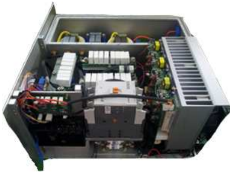
Fig. 16. Picture of developed 20kV, 20kW high-voltage DC power supply.
