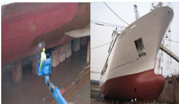
Figure 5: Hull surface condition applied anti-fouling paints of training ship HANBADA
