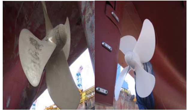
Figure 6: Propeller surface condition applied anti-fouling paints of training ship HANBADA
