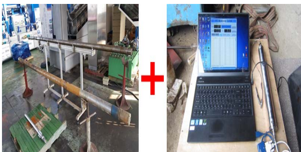
Pressure Core Sampler Data Logging System Figure 1: Main components of reservoir PCS
