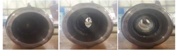
Figure 6: Ball valve operation
