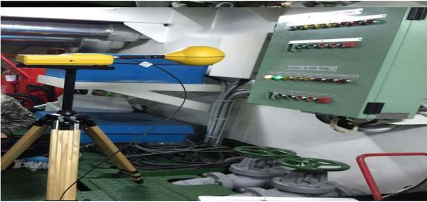
Figure 4: Measurement process of switch board
