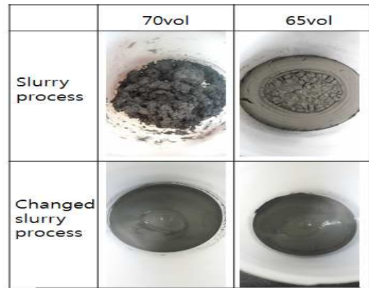
Fig. 3. The image of slurries with the solid loading and the conventional slurry preparation process.
