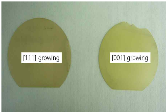
Fig. 5. Bridgman single crystal growing method.
