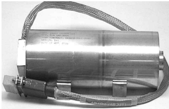
Fig. 1. High-power 1 kW Li/oxychloride reserve battery [1].
