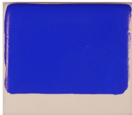
Fig. 2. Thermal stability of blue \text{CoAl}_2\text{O}_4 ceramic ink at 1250°C.
