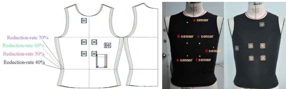
Fig. 1. Example of the smart clothing design for ECG monitoring. Jeong & Yang (2012), p. 41-42.
