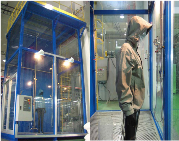
Fig. 2. Developed vertical rain tower system.
