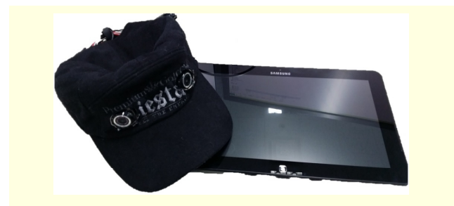
Fig. 3. Hat embedded with two webcams and a smart PC.
