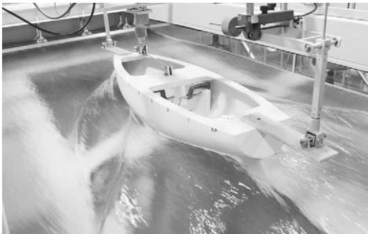
Fig. 18 Wave pattern( \phi=0^\circ , 6knots)
