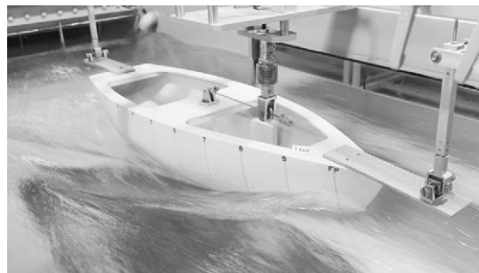
Fig. 13 Wave pattern( \phi=0^\circ , 6knots)
