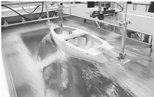
Fig. 23 Wave pattern( \phi=0^\circ , 7knots)
