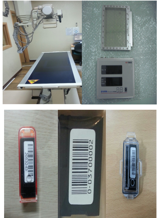
Fig. 1. Device of TLD, PLD and OSLD
