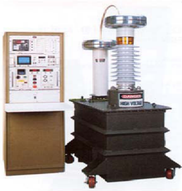
Fig. 2. Experimental equipment of partial discharge.
