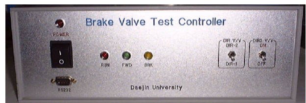
Fig. 6 EHA valve test controller
