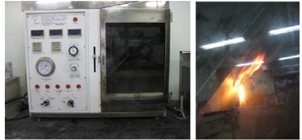
Figure 3: Test apparatus and specimens during the flame-retardant test
