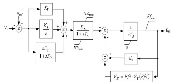
Figure 2: Control block diagram of IEEE type AC8B
