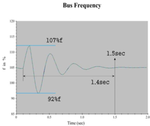
Figure 6: HV feeder frequency when 2 thrusters eliminated with open loop excitation and governor
