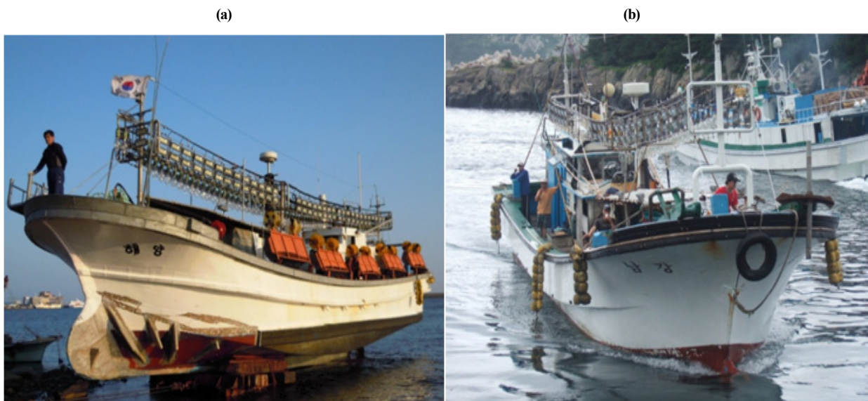
Fig. 1. LED and metal halide luring lamp installed fishing vessel (a:Haeyang, b:Nangang)
