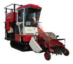
Figure 1. Overview of pick-up type pulse crop harvester.
