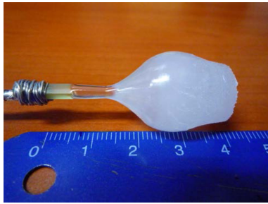
Fig. 1. Photograph of a \text{Li}_6\text{Lu}(\text{BO}_3)_3:\text{Ce}^{3+} scintillator grown by Czochralski method.
