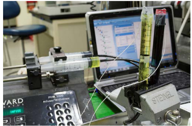
Fig. 3. Experimental setup of CNT nanosheet roll biofuel cell in dynamic flow.
