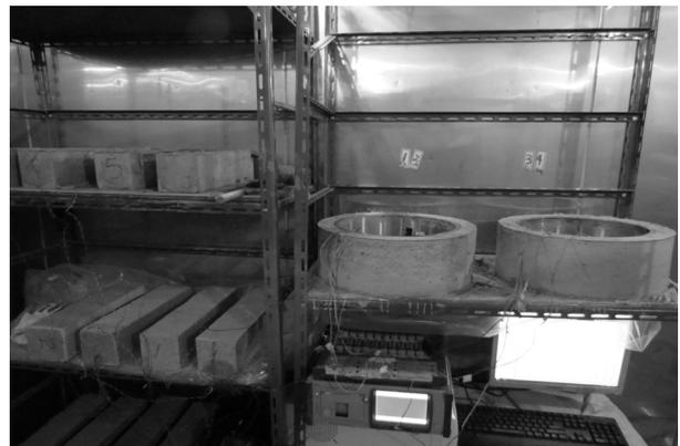
Fig. 3. Ring Test and Shrinkage Test
