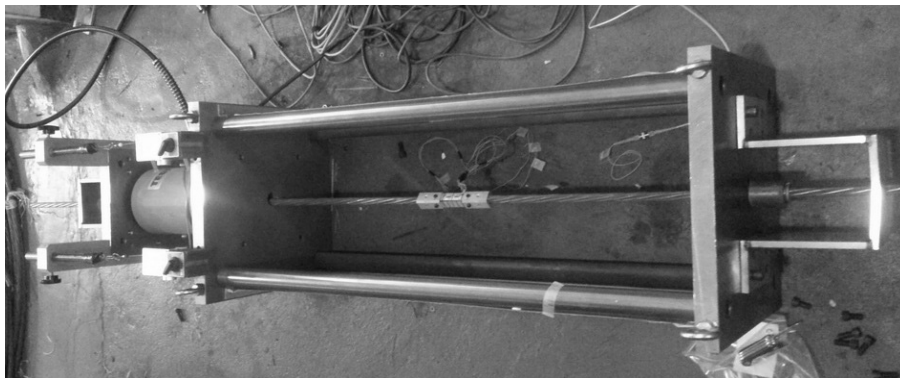
Fig. 8. Experimental Test of Prototype Strand Meter in Laboratory
