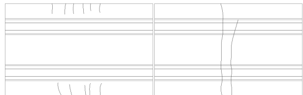
Fig. 15. Crack Patterns (HD1S-1)
