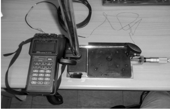
Fig. 8. Equipment for calibration of horizontal displacement sensor
