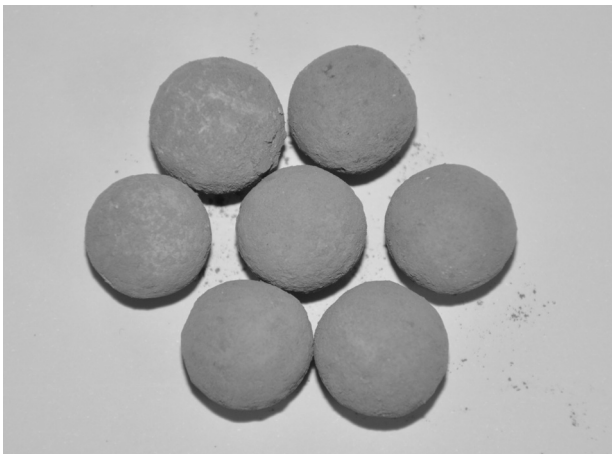
Fig. 1. Spherical-type porous ZSF ceramics, in which natural zeolite and starfish were mixed and calcined with wood flour
