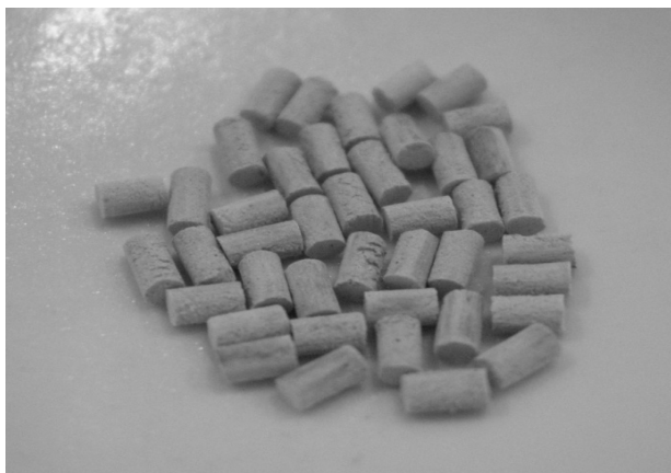
Fig. 1. Pellet-type porous ZSF ceramics, in which natural zeolite and starfish were mixed and calcined with wood flour
