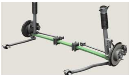
Fig. 1 Geometry of composite leaf spring mounted on rear cross member
