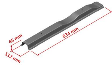
Fig. 2 Shape and dimension of the rear floor cross member
